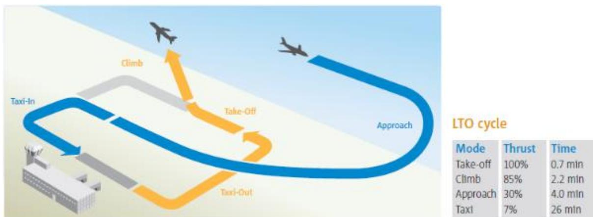
Figure 9 - Standard engine emissions LTO cycle<sup>39</sup>
