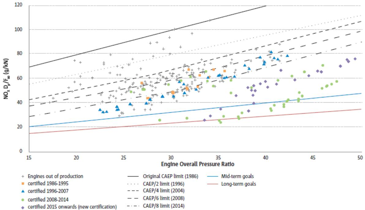
Figure 7. Engine emissions certification data (EASA, 2019)
